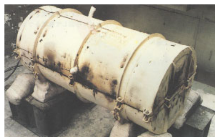
Fig.1 Enriched UF 6 transport package after fireproof test
