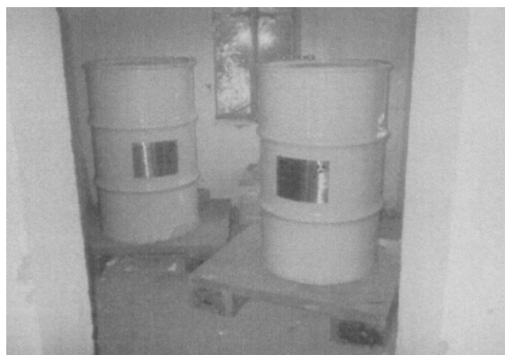
Figure 6: Conditioned disused ^{226}\text{Ra} sources in two 200 L MS drums.
