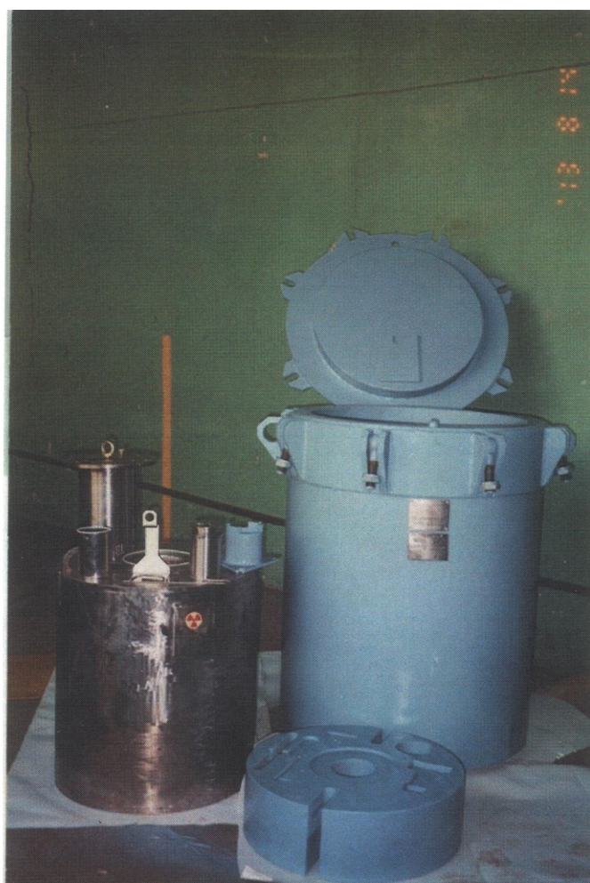
Fig. 2: The transport packaging set UKTIB (U)-96-26M for storage and transport of Co-60 sources, with activity up to 740 TBq (20 kCi) or Cs-137 sources with activity up to 888 TBq (24 kCi)
